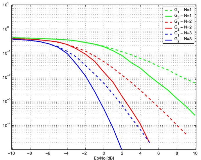
Fig. 2. BER curves of  $\mathcal{G}_1$  and  $\mathcal{G}_2$  in a quasi-static fading channel
