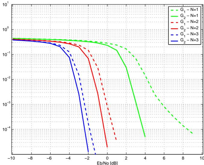
Fig. 3. BER curves of  $\mathcal{G}_1$  and  $\mathcal{G}_2$  in a fully-diversity fading channel
